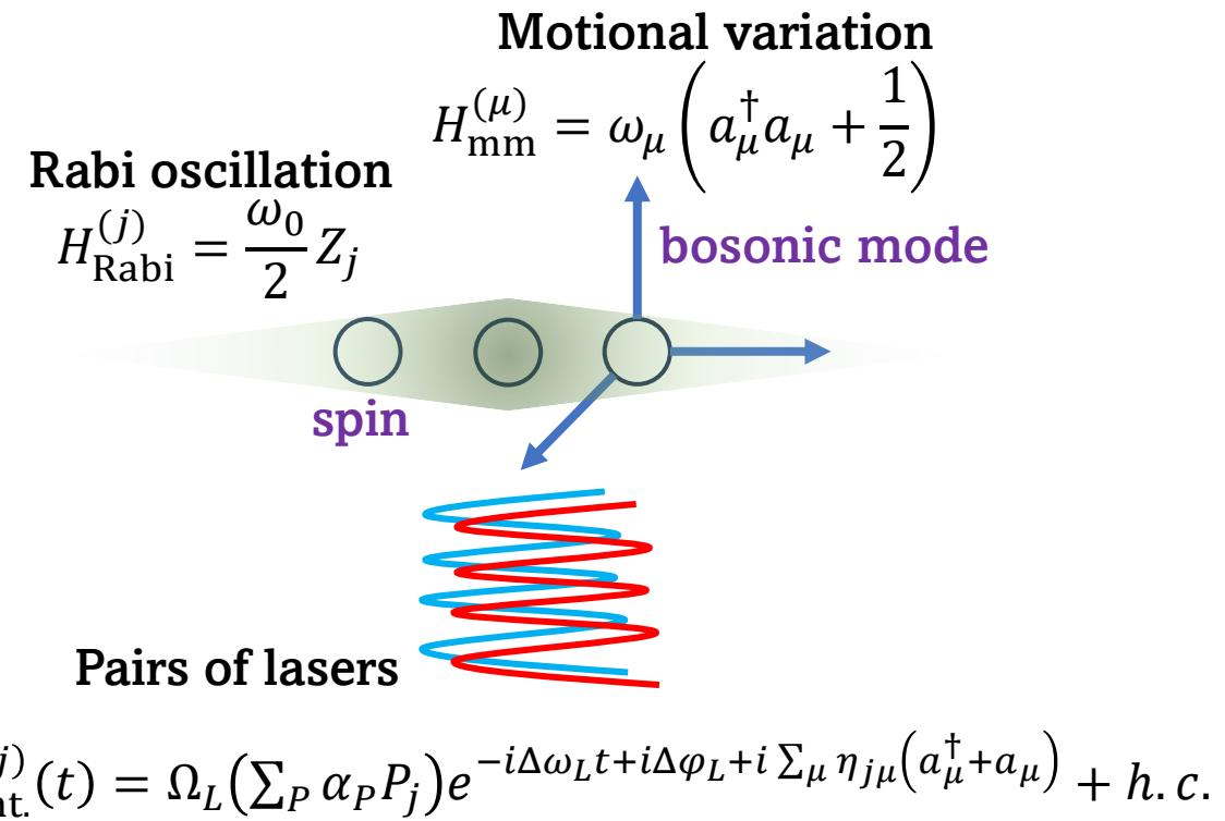
$$H_{\text{int.}}^{(j)}(t) = \Omega_L \left( \sum_P \alpha_P P_j \right) e^{-i\Delta\omega_L t + i\Delta\varphi_L + i \sum_\mu \eta_{j\mu} (a_\mu^\dagger + a_\mu)} + h.c.$$
